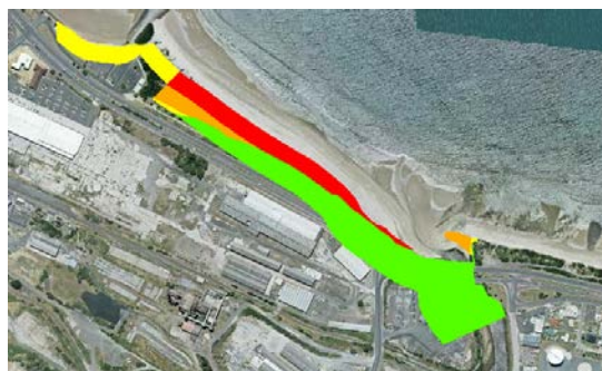
Figure 1: Coastal Erosion Hazard Bands and investigation area (green) at South Burnie
