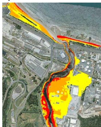
Figure 2: Coastal Inundation Hazard Bands along Emu River near Wivenhoe
